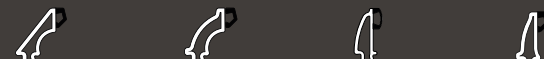
LCW041 28mm Chamf. Bead LSW041 28mm Sculpt Bead LPD083 Flush Sash Bead LCW042 36mm Bead
