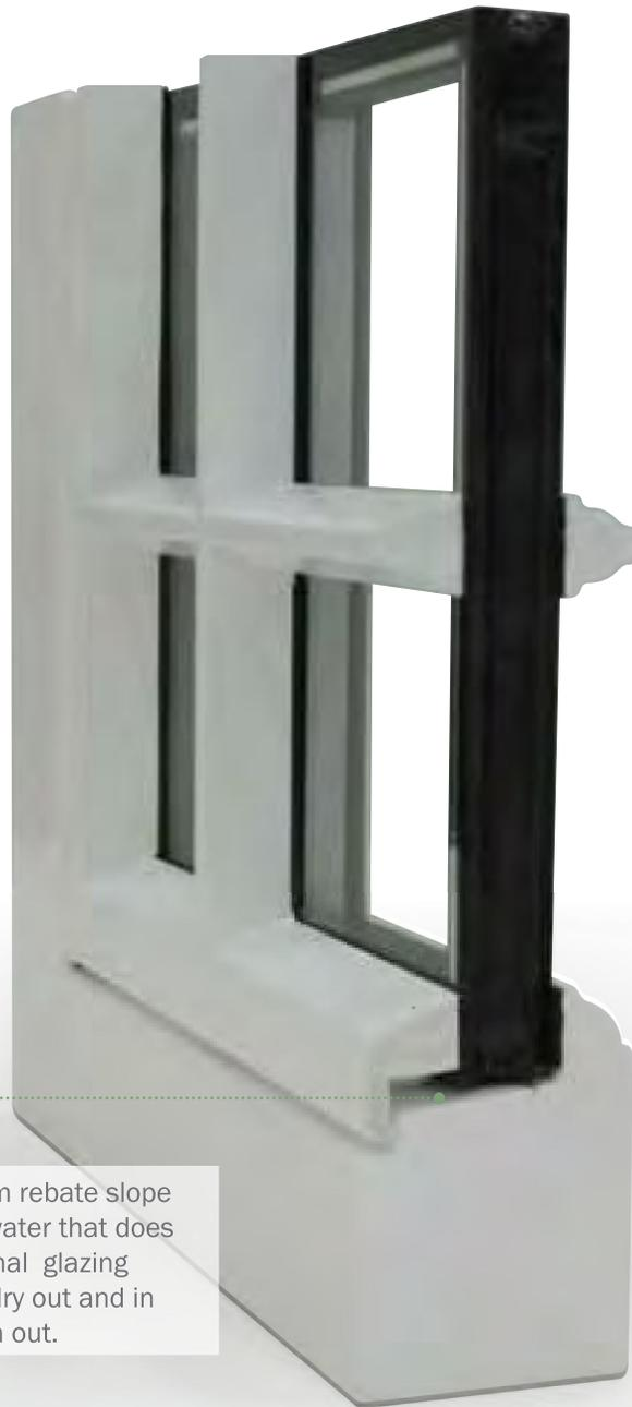
The 7 degree bottom rebate slope ensuring that any water that does penetrate the external glazing seals is allowed to dry out and in extreme cases drain out.
