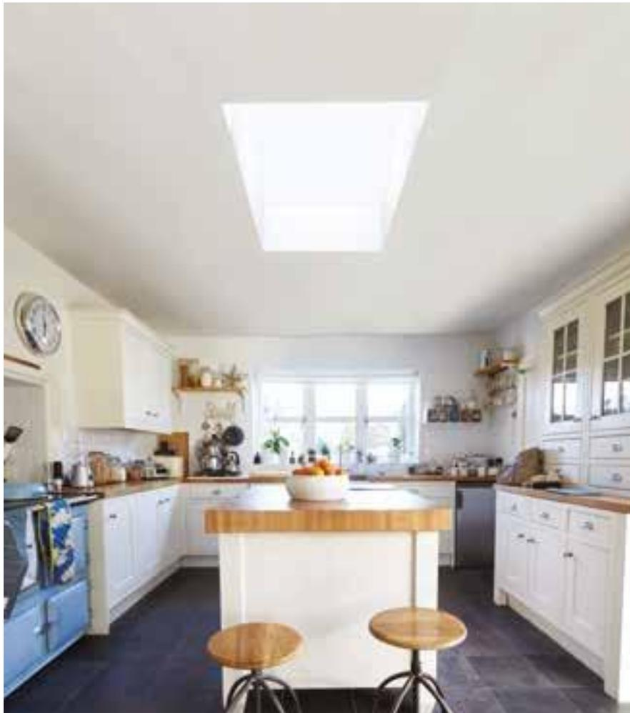
Noise reduction has been built into the design of the Wendland Flat Skylight and can reduce sound by up to 34dB ensuring your room is peaceful and quiet.
